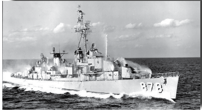
USS Vesole, the picture is unofficially titled “Washdown ‘56”. The purpose was to decontaminate the ship after a nuclear attack. Photo courtesy of Art Pratt.
